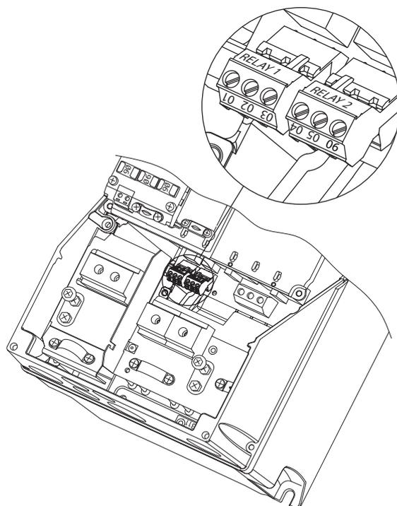
Illustration 6.38 Bornes de raccordement relais
