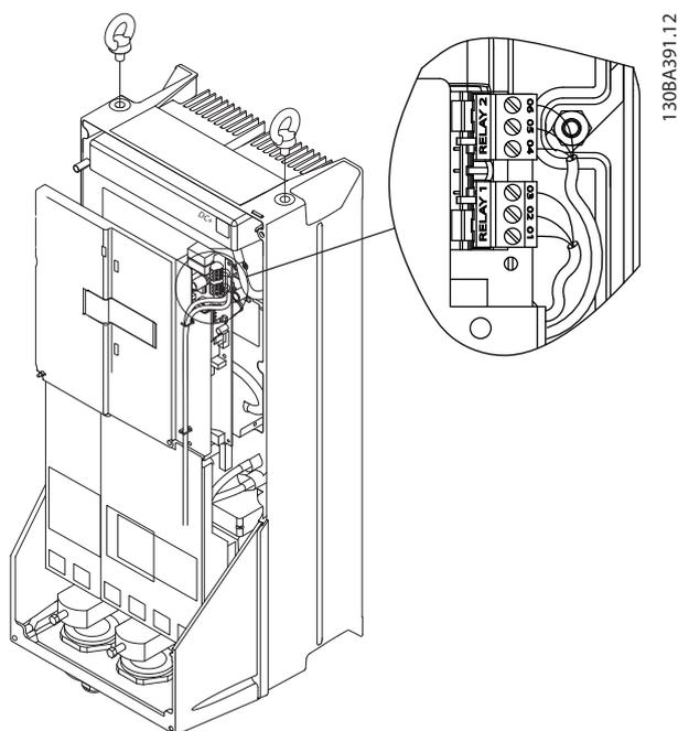
Illustration 6.37 Bornes de raccordement relais
